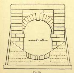
With some modifications to suit local circumstances, they were all made after one type. The lower, or downstream end, is shown by Figs. 16 and 17; the former being an elevation and the latter a longitudinal section. The upstream end is formed with cross wall to obviate the possibility of the current finding a passage behind the masonry.
